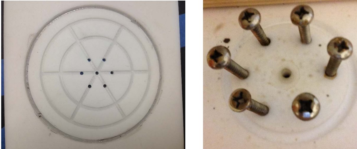
Figure 3. Teflon Column Cap with Drainage Veins and Holes (left) and Stainless Steel Throttling Screws (right)
